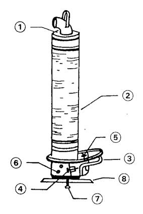
Load adjustment knob (4), this plastic knob will allow the operator to "balance" the load, i.e. to hold the load at a predetermined height without operator assistance. This height may be set at any position depending upon the operator's preference.
